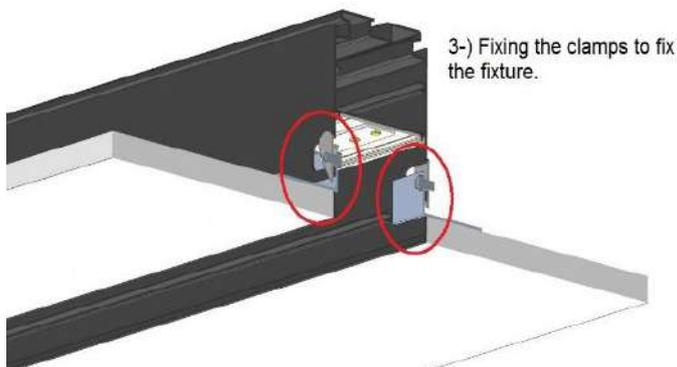
3-) Fixing the clamps to fix the fixture.
