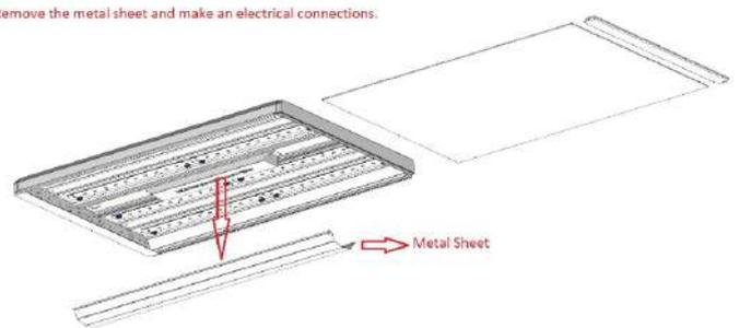
3- Fix the fixture to the ceiling from the fixing points on the body.
