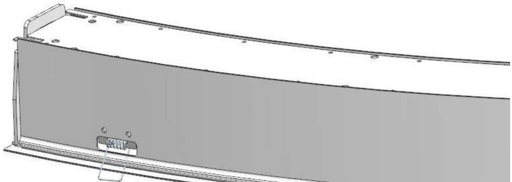
The metal male pins should be inserted into the metal female pins on the opposite side and should be put into place with a rubber mallet.
