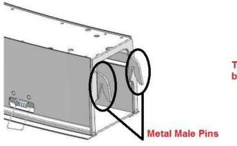
The products must be combined on the floor before mounting on the ceiling!
